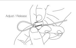
Ensure a minimum 3 inches of tail wire exits the fastener.
