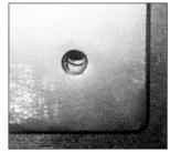
4a. NOT CENTERED If you can see the wall of the duct through any of the corner holes, then it is not centered
