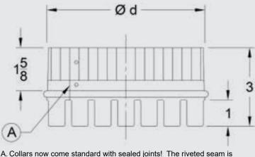
A. Collars now come standard with sealed joints! The riveted seam is sealed with the GreenSeam integral gasket. Unsealed fittings are available upon request.
